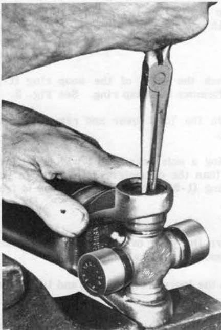
Fig. 2 - Snap Ring Removal
